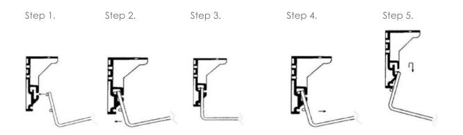
The same bracket is used for both under desk (top) and modesty panel fixing. If extra space is needed, for example to access sockets, the basket may be moved to position 5 whilst access is required.
