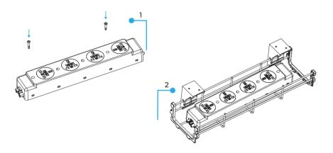
OPTION 2 - FIX THE MODULE INTO A WIRE BASKET Simply place the module into the wire basket.
